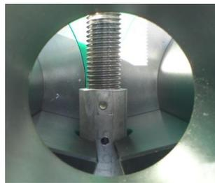
Picture 2. Swaging commence at inspection hole with wire fully visible.
