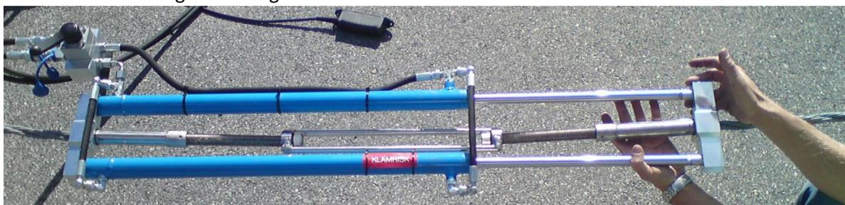
Picture 5. Hydraulic traction device mounted to tensioning unit. Fasten nuts to lock the unit in position.
